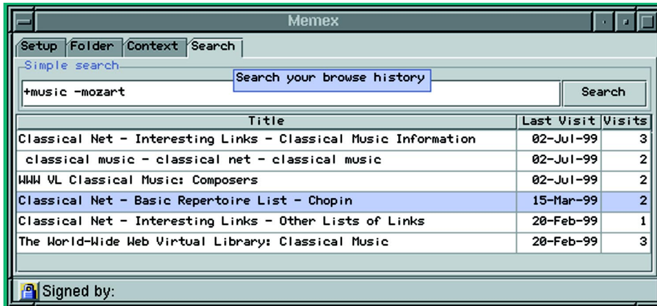
Fig. 2. The Search tab enables boolean and free text search over all archived surfing history. Results can be sorted by various columns.
